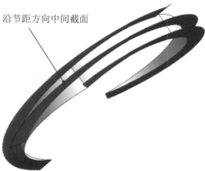
图 4 设计的旋转冲压压缩转子三维进气流道 Fig. 4 Designed three dimensional flow path of the ramr rotor
